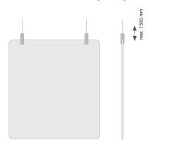
Incl. stainless steel suspension kit for suspension height up to max. 1500 mm Position of the brackets (data in the middle of the bracket): 2 brackets 100 mm indented for aperture width 800 - 1000 mm 2 brackets 200 mm indented for front panel width 1200 - 1800 mm
