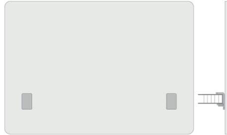
Incl. table fixing for panel thickness 19 to 25 mm
