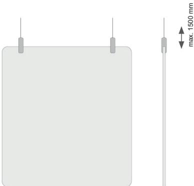
Incl. stainless steel suspension kit for suspension height up to max. 1500 mm
