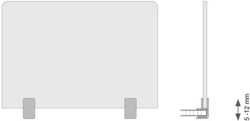
Distance between the top and the table (cable routing) adjustable from 5 to 12 mm
