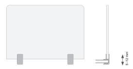
Distance between the top and the table (cable routing) adjustable from 5 to 12 mm Incl. table fixing for panel thickness 19 to 25 mm Position of the brackets (data in the middle of the bracket): 2 brackets 100 mm indented for aperture width 800 - 1000 mm 2 brackets 200 mm indented for front panel width 1200 - 1600 mm 3 Holder 200 mm indented or centred for 1800 mm wide front panel
