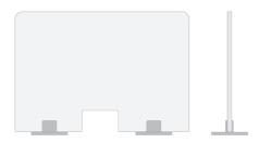
Central cut-out H/W 120/300 mm freely positionable on counter, cupboard or table incl. 2 feet W/D 150/250 mm Position of the feet (data in the middle of the foot): 2 feet 75 mm indented for 600 mm wide front panel 2 feet 100 mm indented for front panel width 800 - 900 mm 2 feet 200 mm indented for front panel widths 1000 - 1600 mm
