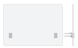
Incl. table fixing for panel thickness 19 to 25 mm
